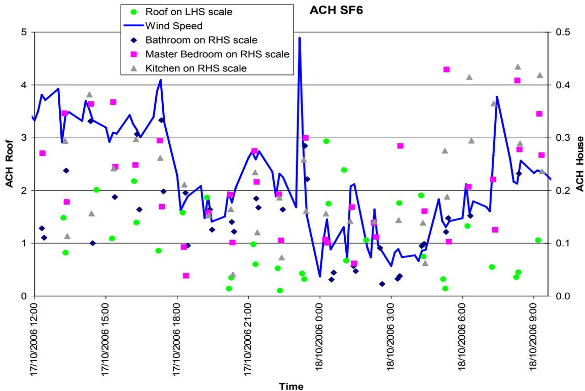
**Figure 10 : Air Change Rate and Wind speed for Lot 602**
