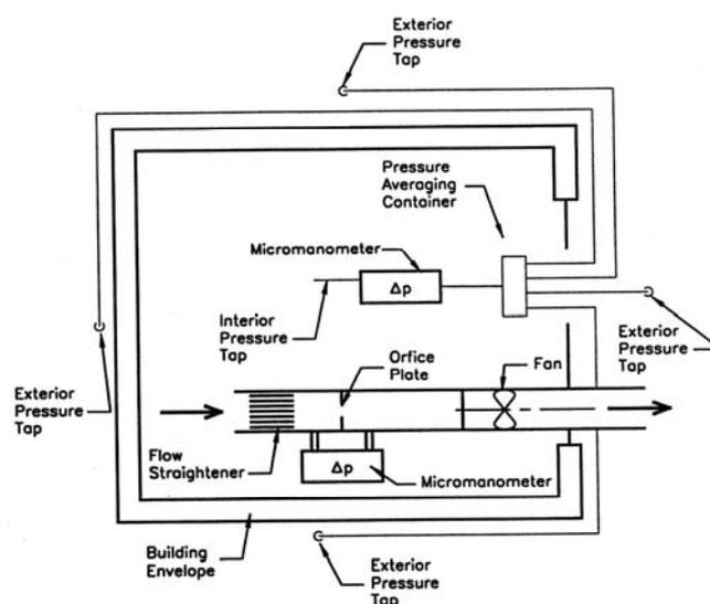
**Figure 3 Pressure Measurements in Blower Door Testing (Proskiw, G. and B. Phillips, 2001)**
