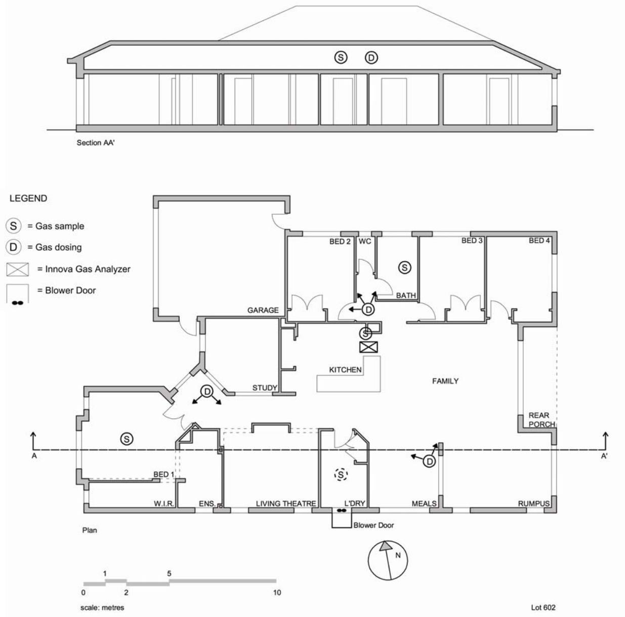
**Figure 6 Section, Plan and Instrument Locations in Lot 602**
