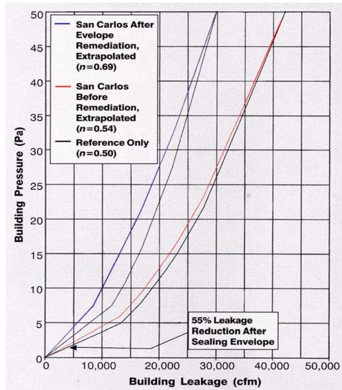
**Figure 1 Air Leakage to Building Pressure Relationship: example (Ask,2003)**
