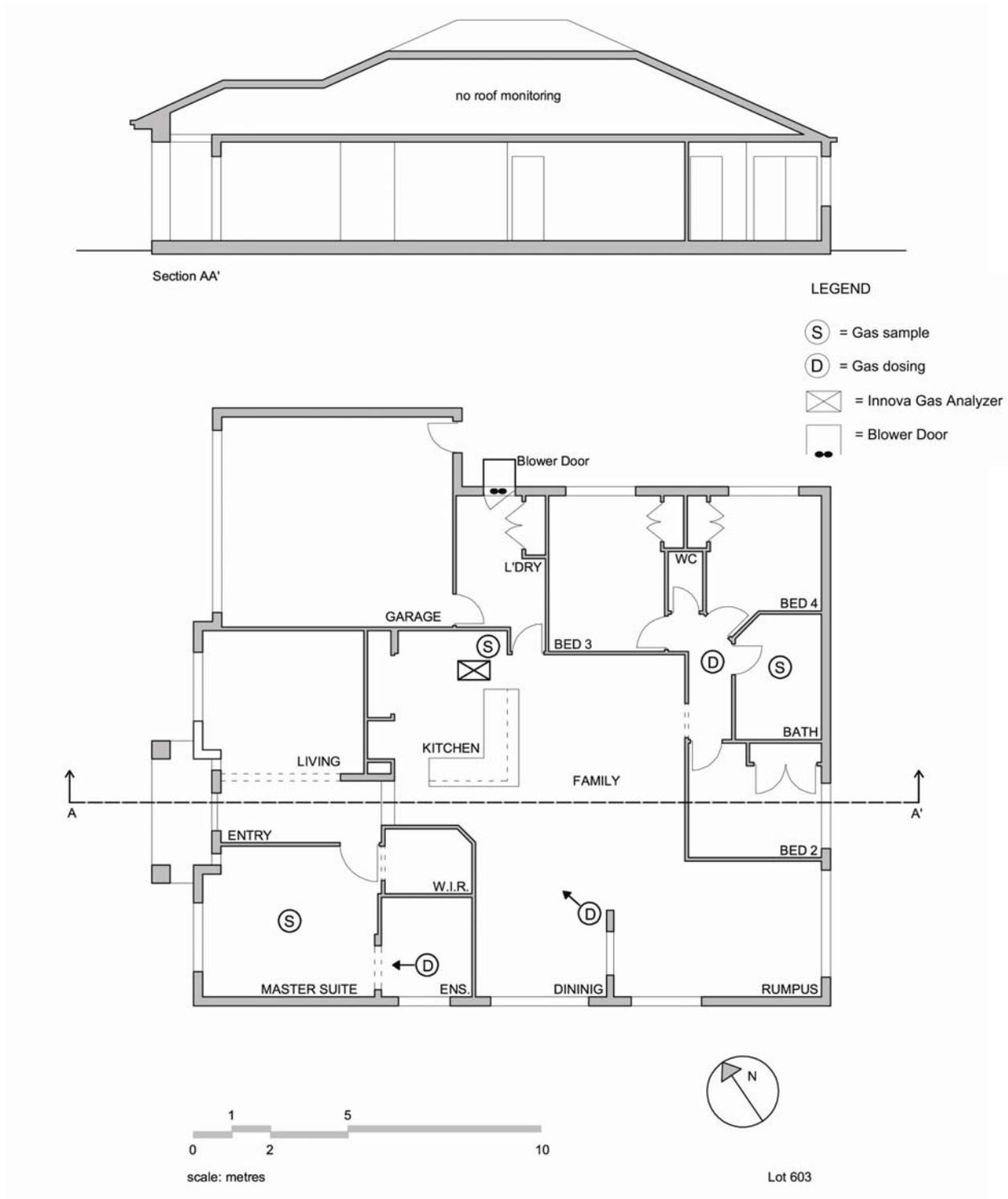
Figure 5 Section, Plan and Instrument Locations in Lot 603
