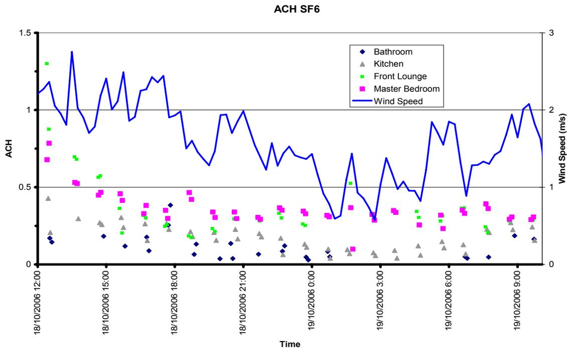
**Figure 11 Air Change Rate and Wind Speed for Lot 603**
