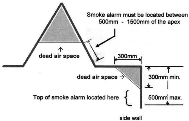
Diagram 3 – Dead air space and proper mounting of smoke alarms on side walls
