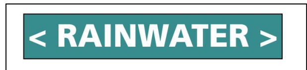
FIGURE 5 - RAINWATER PIPE MARKING
